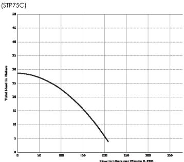
Note: Performance based on pumping solvent (0.78 specific gravity). Pressure is taken at the manifold discharge outlet. Fixed Speed 0.75 HP was powered by Three-Phase, 50 Hz, 415 Volt incoming supply.
