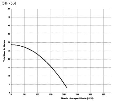
Note: Performance based on pumping solvent (0.78 specific gravity).
